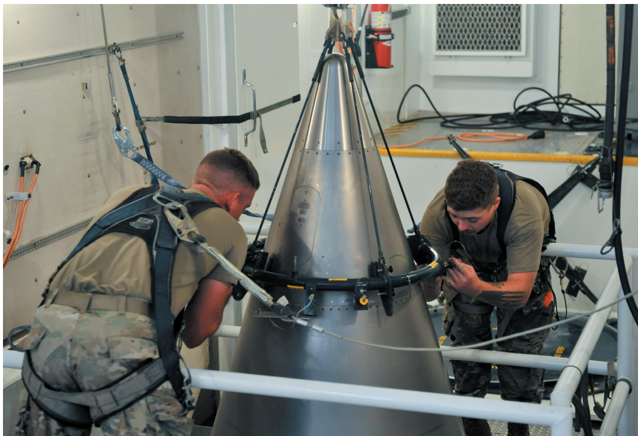
Senior Airman Jacob Deas, left, and Airman 1st Class Jonathan Marrs, right, secure the titanium shroud at the top of a Minuteman III intercontinental ballistic missile on 24 August 2023, at the Bravo 9 silo at Malmstrom Air Force Base in Montana, United States. After the shroud is secured, it is lifted off, revealing the black cone-shaped nuclear warhead inside. (Photo by John Turner/U.S. Air Force via AP/NTB)
